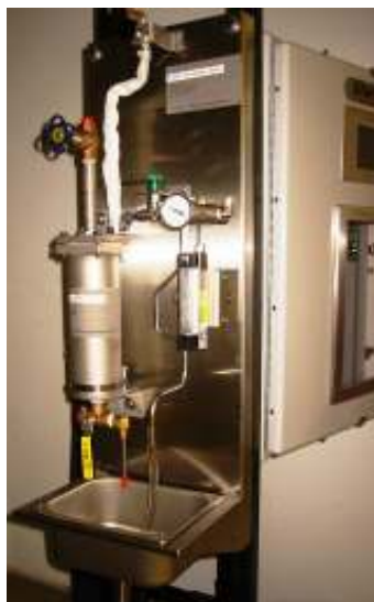
(Heat Exchanger and Sample-Conditioner System)
