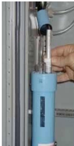
The oxidation reactor of this system does get dirty and clogged because of dissolved salts or suspended solids present in water.
